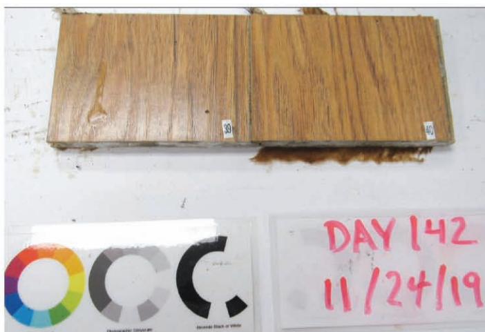
Photo 6. Laminate flooring after 142 days.
