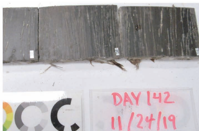
Photo 7. Bamboo flooring with surface cracking after 142 days.
