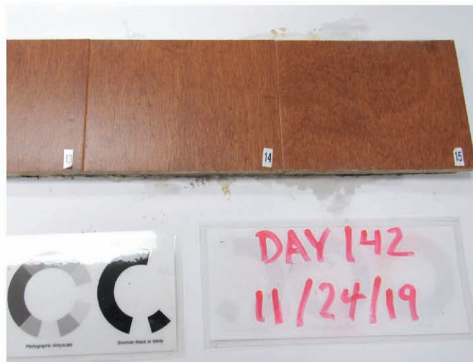
Photo 5. Engineered flooring after 142 days.
