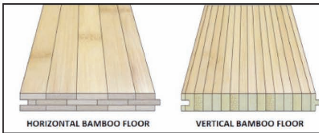
Figure 4. Horizontal and vertical bamboo flooring orientation. Source: BambooFloorCompany.com , a trading name for Kitchner Flooring LTD.
