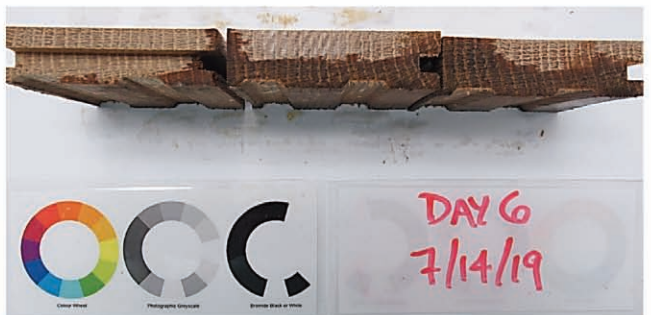
Photo 2. This hardwood flooring exemplar (rift sawn) (Day 6) was the only exemplar that did not exhibit cupping after 142 days exposure to damp concrete.
